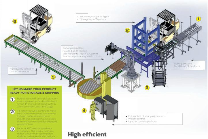
STM offers complete range of palletization systems with high / low level infeed with single / multiple entry for loose bottles and pack layers, able to handle cans, jars, bottles, cartons, bundles and crates.
