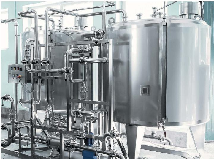
The station preparing solutions and cleaning agents also contains a JAD-type heat exchanger that is designed to transform heat by means of a heating medium in the form of steam.
