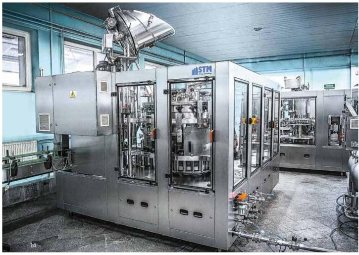
Non-carbonated liquids, Ice Tea, still water, juices, liquids poured into containers at temperatures reaching **up to 88°C.**
